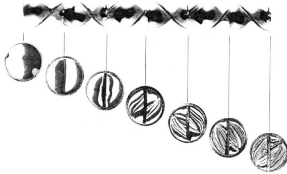
Figure 5 - Upper photo - Laboratory generated laminar mixing example over a six element mixer in laminar flow.
