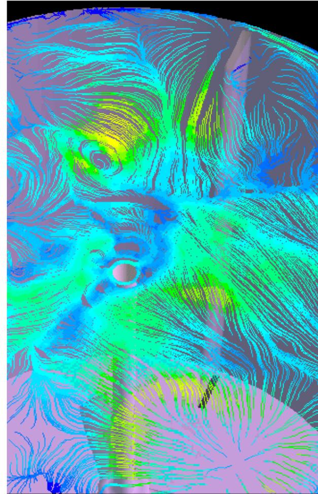
**“Oilflow” lines are pathlines constrained to the surface from which they are released.**
