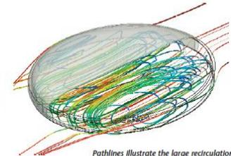
Pathlines illustrate the large recirculation zone underneath a flying Frisbee
