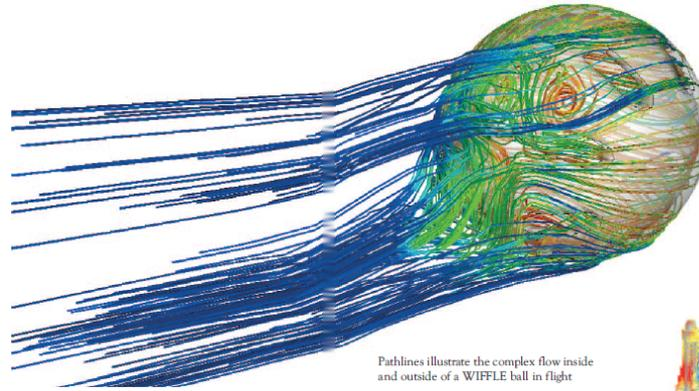
Pathlines illustrate the complex flow inside and outside of a WIFFLE ball in flight
