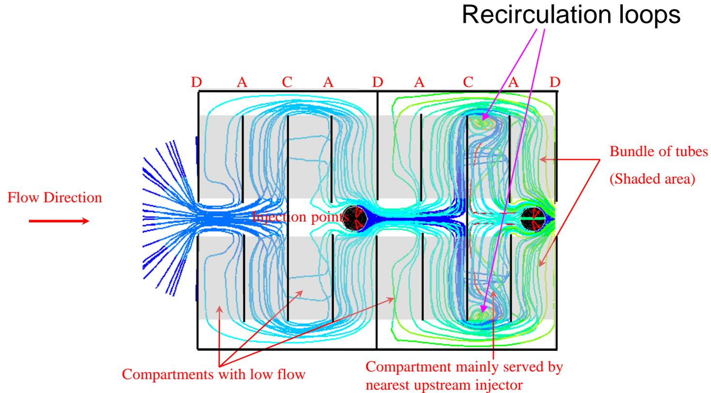
*Non-uniform flow distribution means low efficiency*
