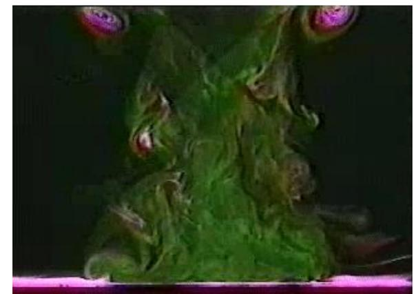
A smoke ring (green) impinges on a plate where it interacts with the slow moving smoke in the boundary layer (pink). The vortex ring stretches and new rings form. The size of the vortex structures decreases over time.
