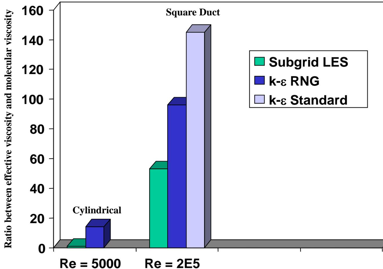
The effective viscosity is lower with the LES model than with the  $k-\epsilon$  models, allowing the vortices in the simulation to become unsteady.
