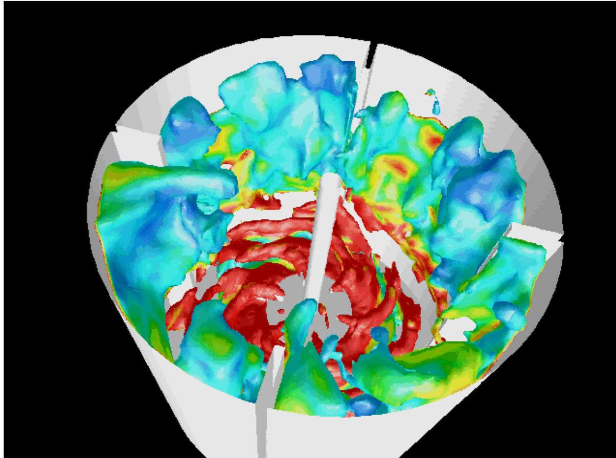
Iso-surface of axial velocity of 0.1m/s. The velocity is directed upwards in the regions enclosed by the iso-surface. The surface is colored by strain rate on a scale of 0 to 100 1/s.
