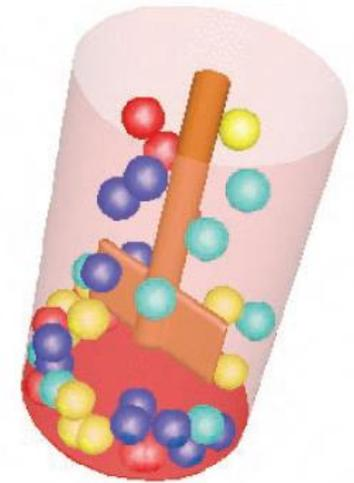
*Balls of different mass continuously injected into a rotating paddle-type mixer*
