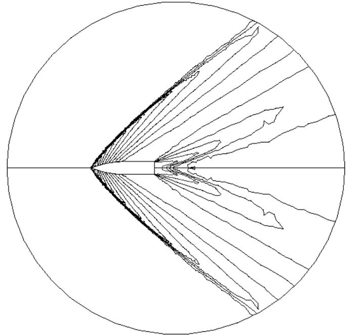
2D planar shell - contours of pressure final grid
