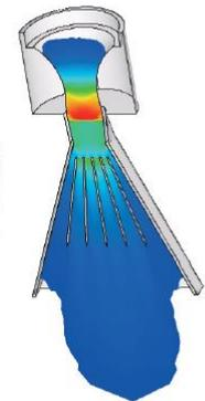
Contours of Mach number in one of the simulated diffuser designs shows choked flow
