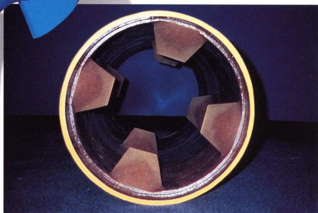
Figure 2 (below). Geometry of the HEV vortex generating tabs.
