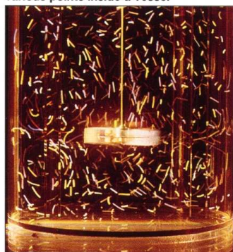
FIGURE 2. Streaklines around a disc-style impeller indicate fluid velocities at various points inside a vessel
