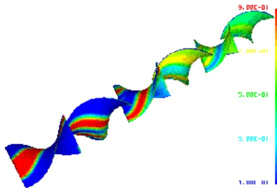
The flow pattern, pressure drop and the mixing characteristics of Kenics™ static mixers are investigated by means of computer simulations. The static mixer consists of a series of alternating left and right hand helical elements.
