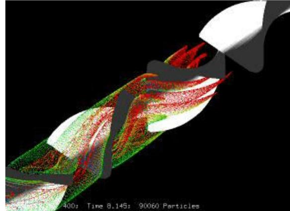
**Figure 9** Particle traces through the Kenics mixer as calculated by HyperTrace.
