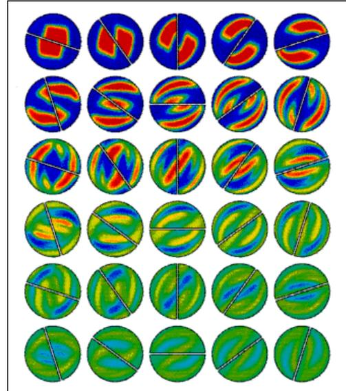
**Figure 7** Concentration profiles in the mixer. Rows one to six show the concentration in elements one to six respectively. Columns one to five show the concentration profiles at 18, 54, 90, 126 and 162 degrees respectively.
