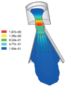
Contours of Mach number in one of the simulated diffuser designs shows choked flow
